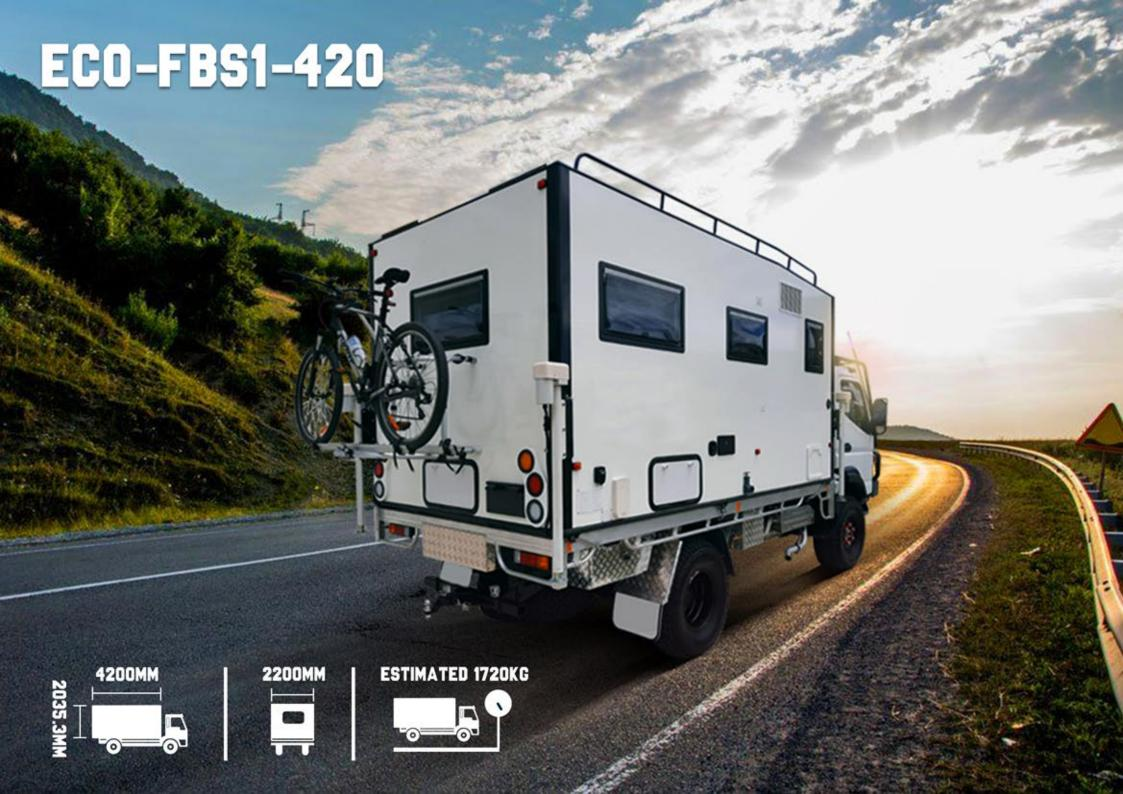
Trailer Body Frame: White Color external Fiberglass + aluminum frame + XPS+ Fiberglass
